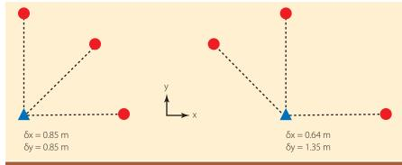
FIGURE 1 Example of the role of measurement geometry. These two examples assume *ranges* are measured to each transmitter and each has an error of 1 meter. Despite the similar geometry, the resulting position errors are quite different.
