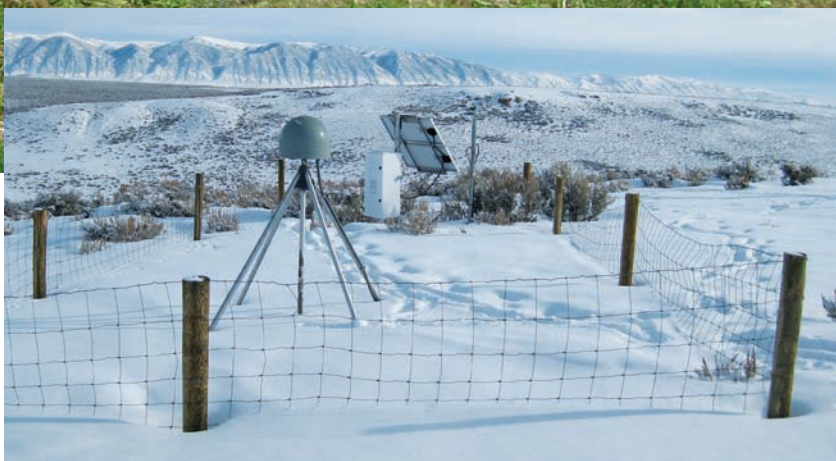
Most PBO sites are operated with banks of batteries that are powered by solar panels, as shown at PBO site P422. Inset: PBO site P101 in Randolph, Utah, which is used to measure snow depth in the winter and vegetation/soil moisture in the spring, summer, and fall. UNAVCO photos
