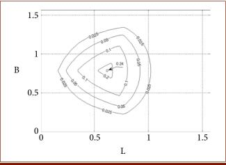
FIGURE 2 Dependence LCA from B and L for interplex modulation
