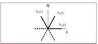
FIGURE 3 Vector diagram of three-component symmetrical MSPM
