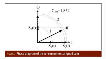
i.e., the power of the third signal, occupying quadrature Q, at the output of the corresponding correlator is larger by 2.62 than the power of the first and the second signals combined on the I quadrature.
