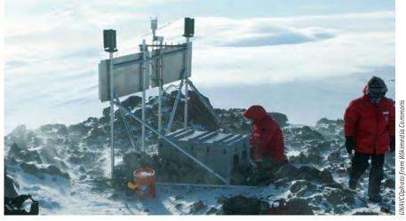
Continuously monitoring GPS station in Antarctica
