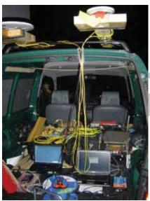
Equipment installation inside the test vehicle
