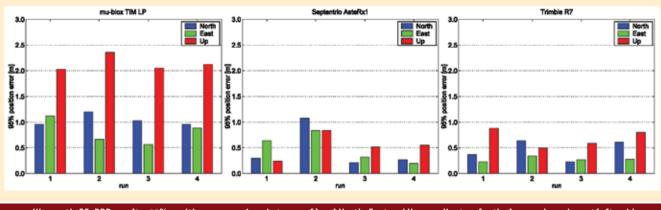
FIGURE 4 Kinematic SF-PPP results: 95% position errors, given in terms of local North, East and Up coordinates, for the low-end receiver at left, midrange receiver in the middle, and high-end receiver at right.
