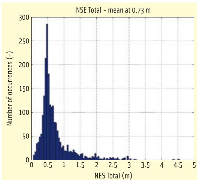
FIGURE 3 Navigation System Errors, Jan. 23, 2006, flight trials
