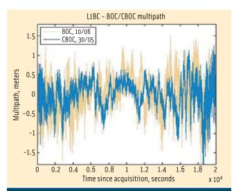
FIGURE 4 Multipath time series for L1BC for June 10, when BOC(1,1) was transmitted (results in light brown ), are compared to May 30 , when CBOC was transmitted (results in blue, comparison by method [a] described in article text).
