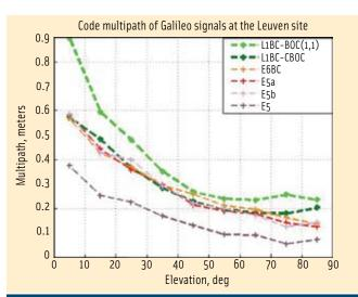
FIGURE 3 Standard deviation of code multipath for Galileo signals transmitted by GIOVE-B. The two thicker lines indicate L1BC modulations: BOC(1,1) in light green and CBOC in dark green.
