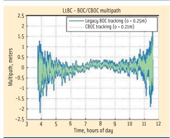
FIGURE 5 Simultaneous multipath time series of BOC(1,1) (blue) and CBOC (light green) obtained by the tracking of CBOC in two modes (comparison method [b]) for May 08 2008.
