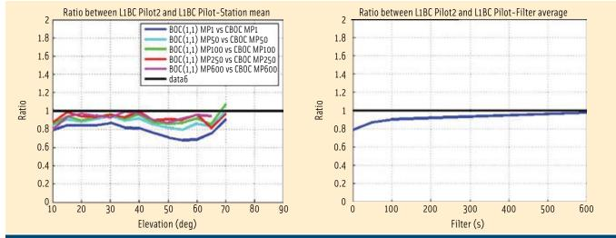
FIGURE 6 Left side: ratio of the range error STD ratio of CBOC/BOC(1,1) as a function of the elevation angle for various filtering windows (1, 50, 100, 250, and 600 seconds). Right side: total standard deviation as a function of the filtering window.
