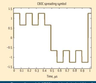
FIGURE 1 The spreading symbol of CBOC is made by algebraic addition of BOC(1,1) and BOC(6,1) spreading symbols.
