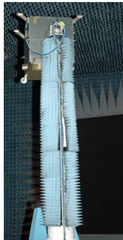
Configuration with two satellites in anechoic chamber (2006 CNES campaign)
