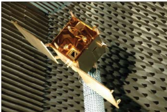
PRISMA radioelectrical mock-ups with S-band helix antennas in CNES anechoic chamber (2007 campaign)
