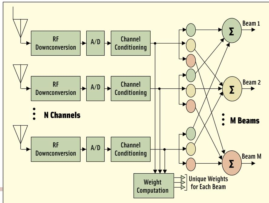
FIGURE 2 Multiple Output Beamformer
