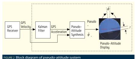
ity measurements than by simply differentiating GPS positions. The acceleration vector  $a_g$  has to be derived externally because in many commercially available GPS receivers, as with the receiver used for this demonstration, acceleration states are not provided in the receiver navigation solution.
