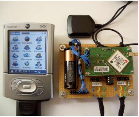
Handheld attitude indicator consisting of PDA and GPS receiver board.
