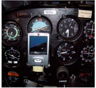
CockpitsetupwithGPSreceivermountedondashboard(left) and pseudo-attitude display side-by-side with artificial horizon (above).
