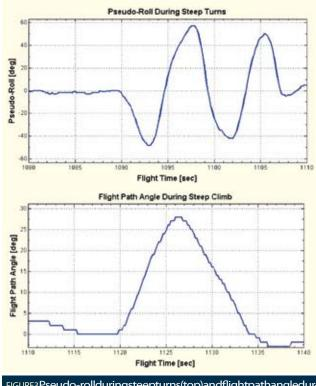
FIGURE3Pseudo-rollduringsteepturns(top)andflightpathangleduring steep climb (bottom)
