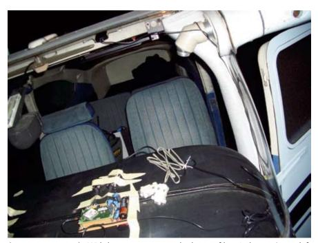
With the antennamounted at the top of the windscreen (upper left in photo), the GPS pseudo-attitude system (visible on dash) was able to receive signals from almost all satellites visible in the sky.
